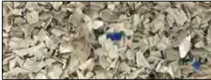
Figure 13: Unwashed HDPE flakes entering the washing process
