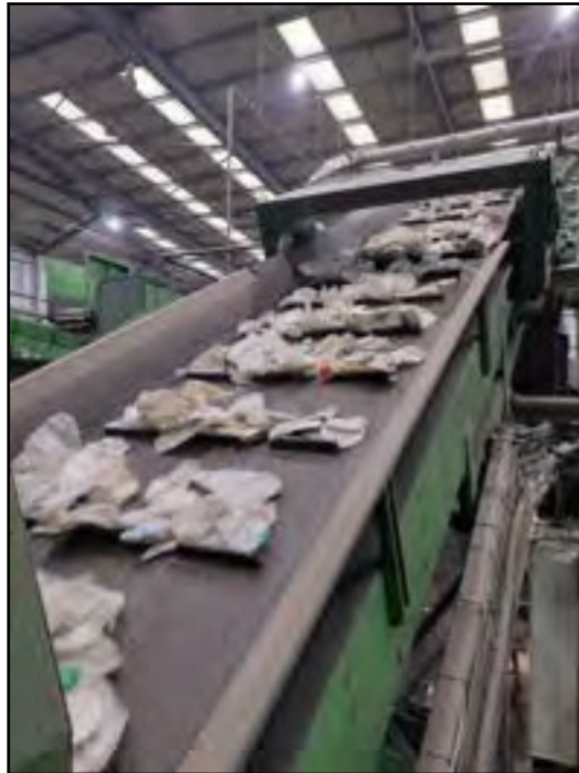
Figure 8: HDPE articles following automated and manual sorting step, which is sampled frequently to determine its composition
