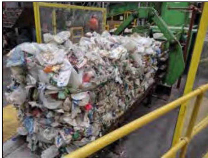
Figure 7: Rejected material from the sorting process, rich in non-food HDPE items
